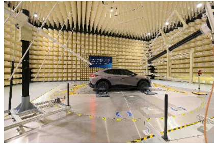
The Electromagnetic Compatibility Laboratory of Volkswagen Group China Technology Company: Testing the reliability of vehicle electronic systems
