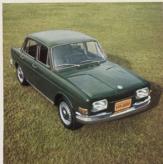
VW 411: Air-cooled, four cylinder, horizontally opposed, rear engine; engine displacement 102.5 cu. in.; 76 SAE bhp engine at 5,000 rpm; independent wheel suspension; Mc Pherson suspension in front; trailing A-arms and double-jointed axle in rear; maximum speed 90 mph; unit body construction; two or four doors. Luxury "L" model available on request. Can also be delivered with automatic transmission.
