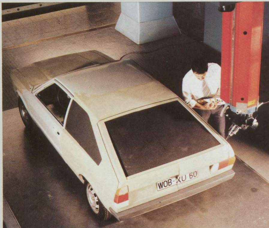
A styling model in the body contour sensing rig
