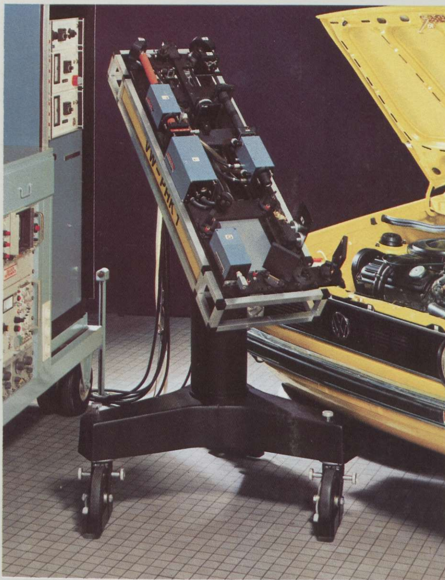
The hologram camera developed by VW can even make sounds visible
