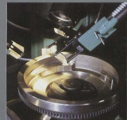
(Flywheel) optoelectronic surface examination
