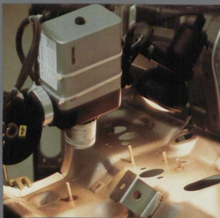
Television camera and microcomputer checking a body part for completeness.
