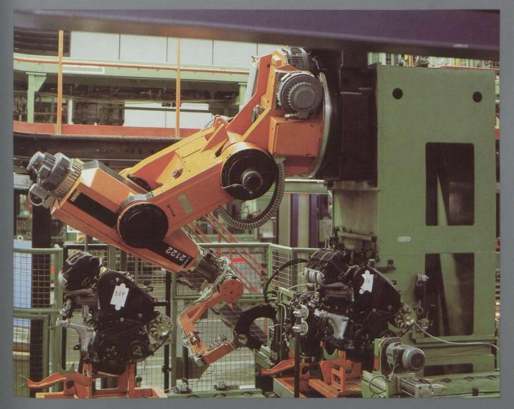
Attaching the engine to the subframe in the power block line
