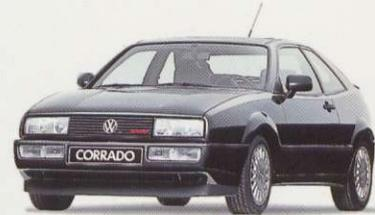
The performance of the VW Corrado matches its sporty appearance. Its 1.8 litre four-cylinder engine with G-supercharger produces 160 bhp.
