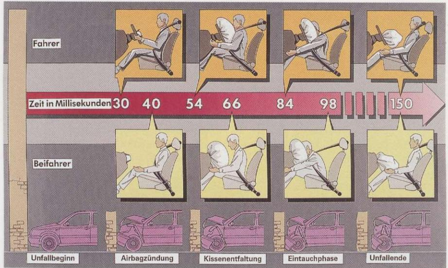
How the dual-airbag system operates
