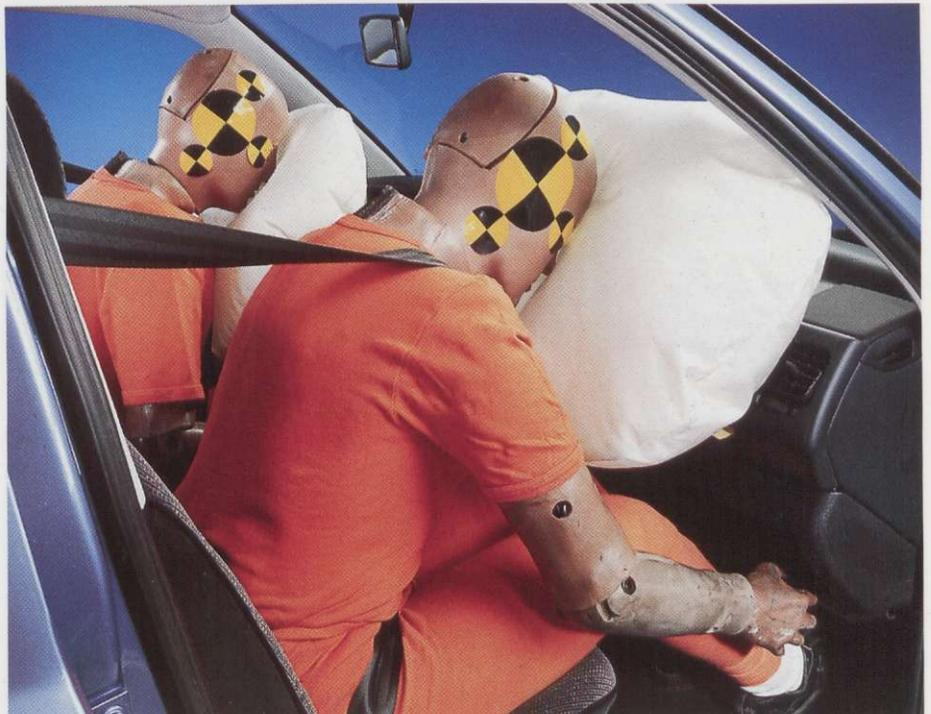
*New standards in safety – airbags for driver and front passenger in the Golf, Vento and Passat*
