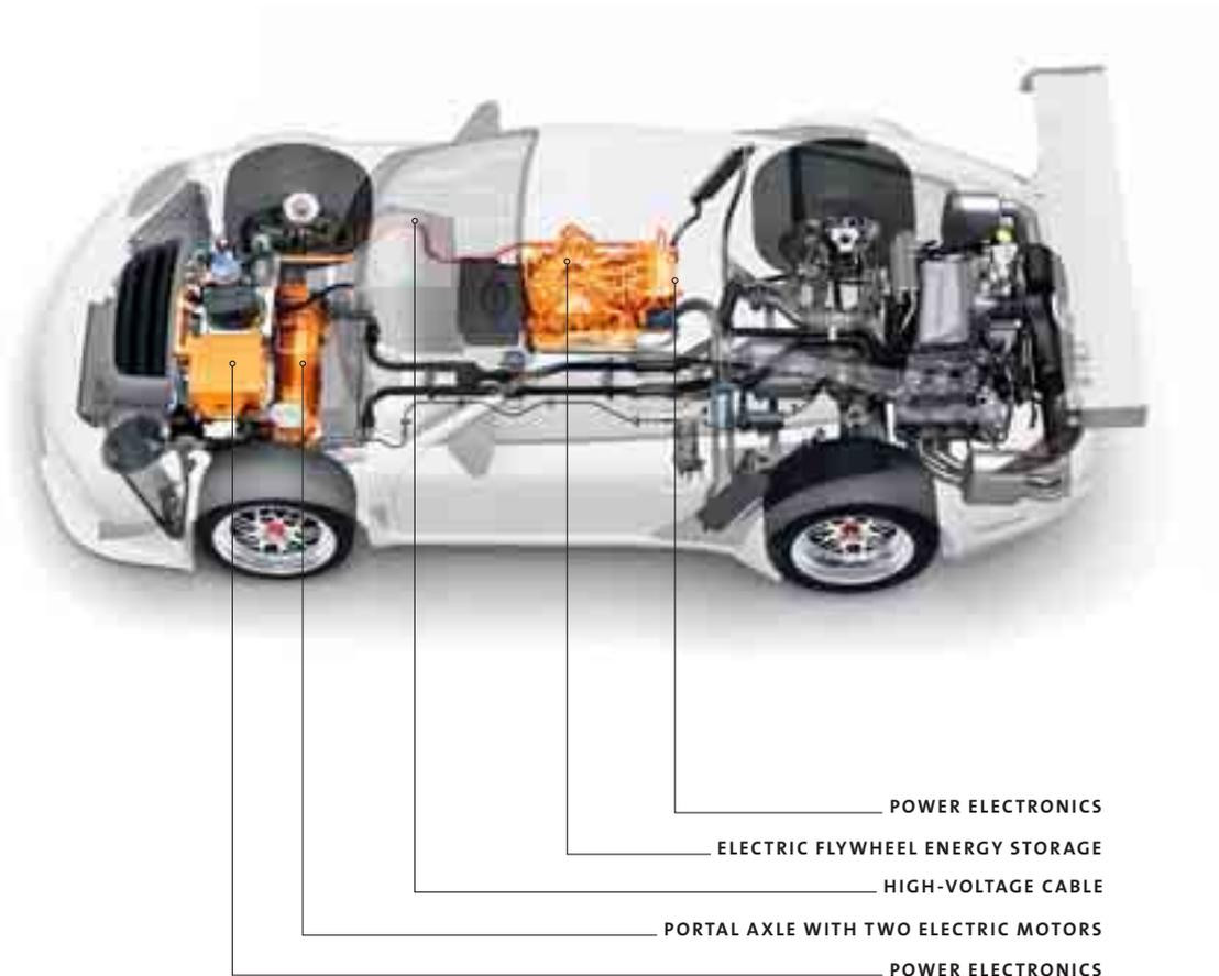
**HIGHER EFFICIENCY, LOWER CONSUMPTION –** Porsche has long been committed to electromobility as a way of protecting the environment and resources. The concept of Porsche Intelligent Performance is based on increasing efficiency while reducing consumption. The hybrid system in the 911 GT3 R Hybrid (pictured on the left) was specially developed for racing. The electrically powered front axle, which does not require a differential lock, will go into series production by 2013 at the latest.
