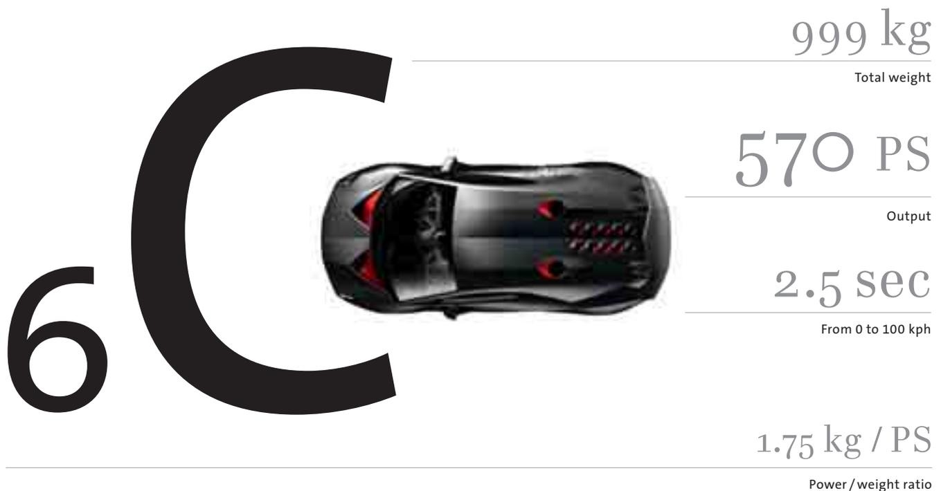
**THE "LIGHT" FUTURE** – With the pioneering Sesto Elemento ("Sixth Element"), Lamborghini engineers undercut the 1,000 kilogram mark for a thoroughbred sports car. The high-performance 570 PS model weighs in at just 999 kilograms, thanks to carbon fiber materials in the vehicle structure, the body outer skin and even in the chassis and the drivetrain.
